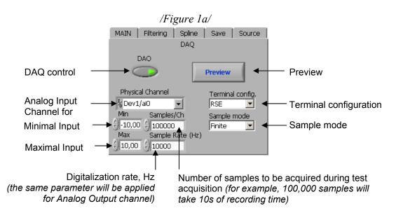
Press Preview button to view the signal at the selected channel in separate window (Fig. 1b). /*Figure 1b*/
