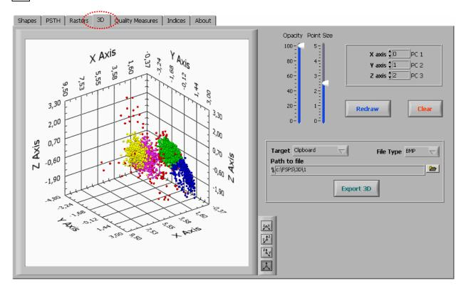
Shows the 3D Scatter Plot of the first three PCs accumulating maximal variance. Other PCs can be viewed by selecting their numbers using the controls in the top right corner.
