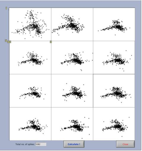
Scatter-plots of Principal Component 1 vs. Principal Component 2 for each spike waveform extracted automatically from the dataset. 2D spatial distribution of PCs gives the experimenter an instant view of the maths of the recorded dataset and the consistency of trials within the experimental "Condition".
