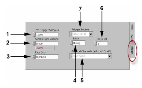
1 – The number of pre-triggered samples. In this specific case 10000 samples equal 1 s (Digitalization rate specified in 3 is 10000 samples/s);
