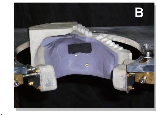
This system allows some small head movements, thus forcing us to directly mount the microelectrode holder to the chamber (fragment C).
