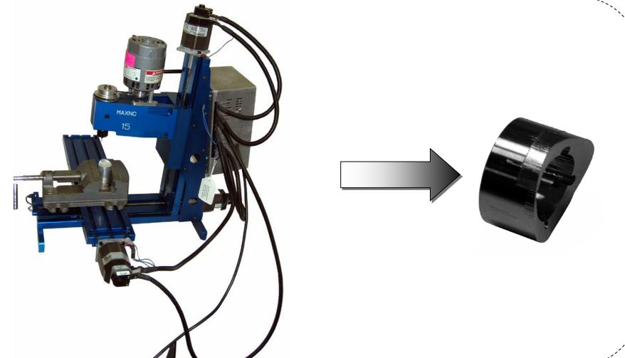
The head fixation system was the most critical part of our implant. After several attempts to use titanium head holders implanted on the skull (fragment A), we decided to build a non-invasive head holder restraining the head by means of shell-like structure (fragment B).
