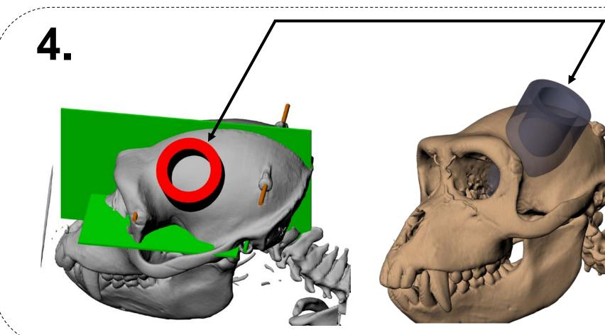
Our recording chambers were made of medical grade titanium and were perfectly fitting the skull surface curvature to maximize the contact surface. For this purpose, the part adjacent to the skull was cut out from the digital 3D mesh of outer skull surface by using the 'Rhinoceros 2.0' software.
